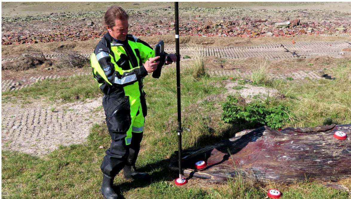
Figuur 3. Inmeten van de Ground Control Points. Foto: Martin Baptist, Wageningen Marine Research, 28-04-2021.
